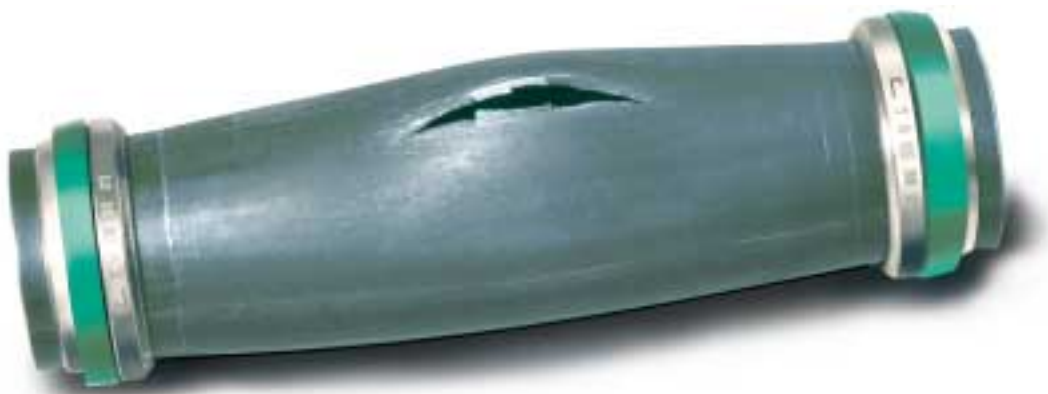
Destructive testing with 28x2 carbon steel tube The tube burst at 650 bar without any leakages or sweating from the sealing points
