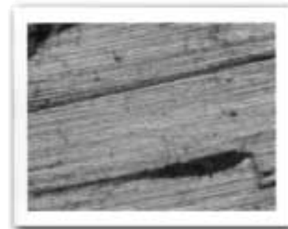
SEALING POINT 3 – 24° CONE
