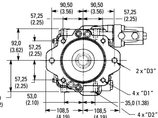
SAE "C" rear mounting. Mounting pad is machined to accept AS568-159 O-ring. Mounting pad is connected to pump case and must be sealed.
