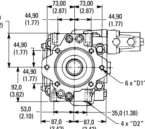
SAE "B" rear mounting. Mounting pad is machined to accept AS568-155 O-ring. Mounting pad is connected to pump case and must be sealed.
