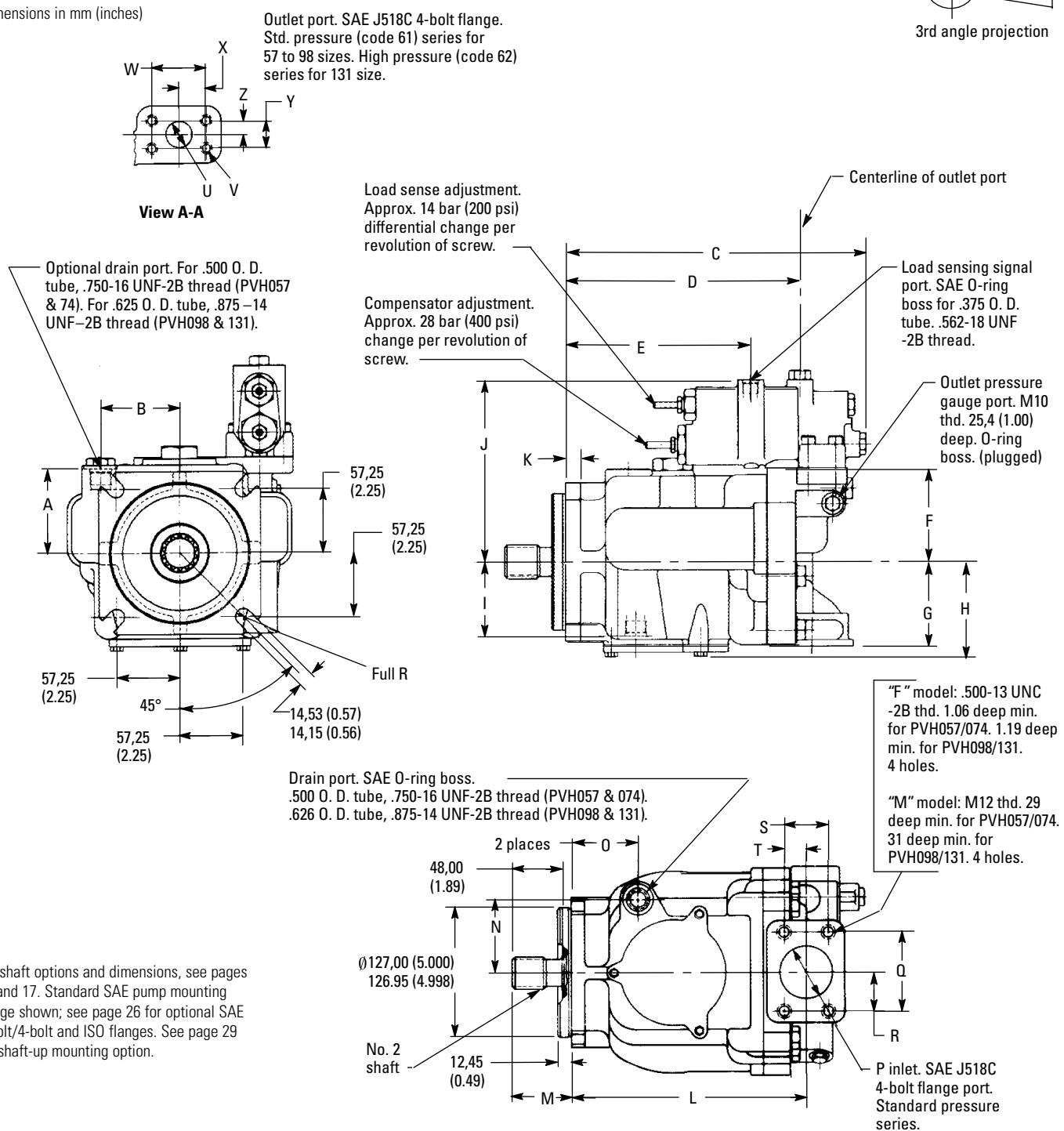
For shaft options and dimensions, see pages 16 and 17. Standard SAE pump mounting flange shown; see page 26 for optional SAE 2-bolt/4-bolt and ISO flanges. See page 29 for shaft-up mounting option.
