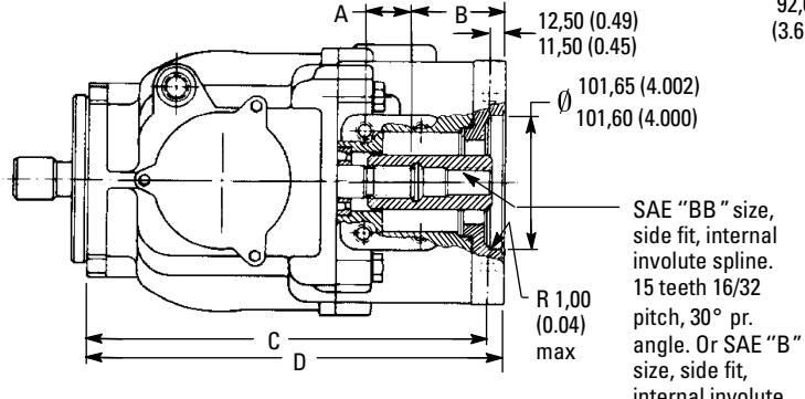
Thru-drive pumps must have support located by dimension "C".
