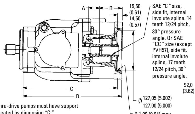
Thru-drive pumps must have support located by dimension "C".
