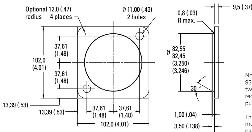
Note: When cover (part number 939790) is ordered as a separate part, two screws (part number 170177) are required to attach the cover to the pump's rear mounting flange.
