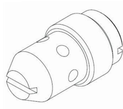
*They are flow control valves, two ways, pressure compensated and with fixed orifice. Flow setting is preadjusted through the calibrated orifice drilled on the compensator piston and is kept constant from 'B' to 'A' regardless of the  $\Delta p$  between port 'B' to 'A'. On the opposite direction the flow is restricted (not pressure compensated) according to the orifice size.*
